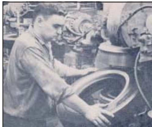
FINISH: Buffing and cleaning the tire's white sidewall.
